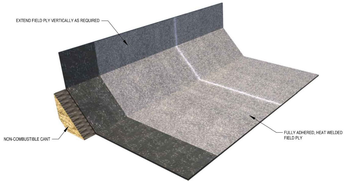
Figure 3.1.1c Fully Adhered, Heat Welded Vapor Retarder Termination at Wall/Curb With Cant
