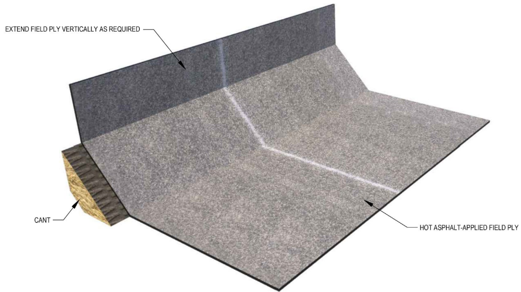
Figure 3.4a Hot Asphalt-Applied Vapor Retarder Termination at Wall/Curb With Cant
