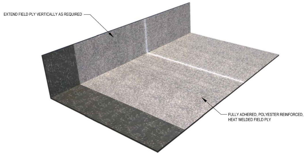
Figure 3.1.1a Fully Adhered, Heat Welded Vapor Retarder Termination at Wall/Curb Without Cant
