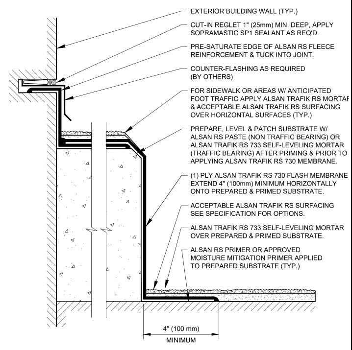
SOPREMA DETAIL DRAWINGS: REFER TO SOPREMA AND OTHER RELATED PUBLISHED DOCUMENTATION, PRODUCT DATA SHEETS (PDS) AND SAFETY DATA SHEETS (SDS) FOR ADDITIONAL INFORMATION. ALL DETAIL DRAWINGS AND RELATED INSTALLATION GUIDELINES ARE PROVIDED BY SOPREMA FOR THE SOLE PURPOSE OF ISSUING A SOPREMA WARRANTY. ACCORDINGLY, THE DETAIL DRAWINGS ARE NOT OFFERED, AND SHOULD NOT BE CONSIDERED, AS A SUBSTITUTE FOR PROFESSIONAL DESIGN SERVICES.
