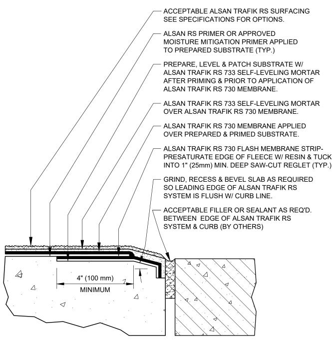
SOPREMA DETAIL DRAWINGS: REFER TO SOPREMA AND OTHER RELATED PUBLISHED DOCUMENTATION, PRODUCT DATA SHEETS (PDS) AND SAFETY DATA SHEETS (SDS) FOR ADDITIONAL INFORMATION. ALL DETAIL DRAWINGS AND RELATED INSTALLATION GUIDELINES ARE PROVIDED BY SOPREMA FOR THE SOLE PURPOSE OF ISSUING A SOPREMA WARRANTY. ACCORDINGLY, THE DETAIL DRAWINGS ARE NOT OFFERED, AND SHOULD NOT BE CONSIDERED, AS A SUBSTITUTE FOR PROFESSIONAL DESIGN SERVICES.
