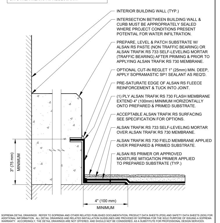
PROJECT: DRAWN BY: SOPREMA TECHNICAL SUPPORT, DWALDRON NO. **REVISION**: DATE: ALSAN TRAFIK RS FULLY REINFORCED US CORPORATE ADDRESS DRAWING NUMBER: 310 QUADRAL DRIVE DATE: 1-15-2024 **WATERPROOFING & SURFACING** WADSWORTH, OHIO 44281 US.RTR.05.C01 GARAGE INTERIOR CURB FLASHING SCALE: Tel:330.334.0066
