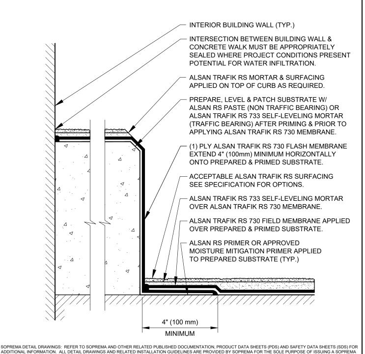
PROJECT: DRAWN BY: SOPREMA TECHNICAL SUPPORT, DWALDRON NO. **REVISION**: DATE: ALSAN TRAFIK RS FULLY REINFORCED US CORPORATE ADDRESS DRAWING NUMBER: 310 QUADRAL DRIVE DATE: 1-15-2024 **WATERPROOFING & SURFACING** WADSWORTH, OHIO 44281 US.RTR.05.C02 **GARAGE INTERIOR CURB/SIDEWALK** SCALE: Tel:330.334.0066
