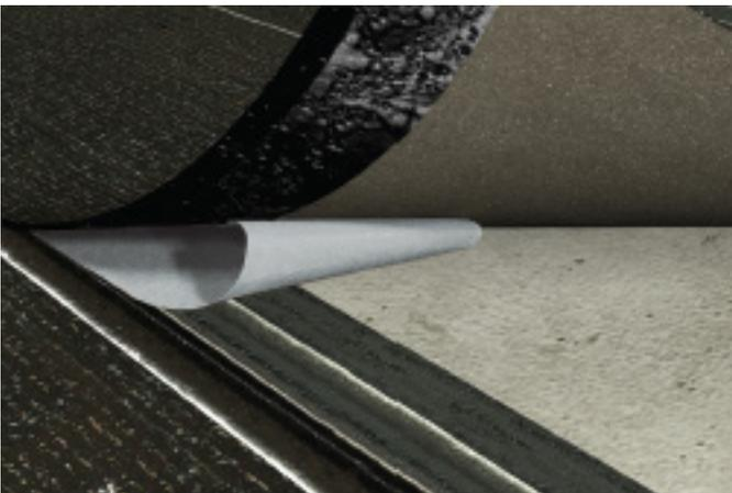
During installation, ensure the DUO SELVEDGE side-laps are maintained clean and dry with the self-adhesive release film applied. To seal the side laps, remove the self-adhesive release film from the DUO SELVEDGE side lap and apply pressure with a weighted roller. Heat-weld the remaining outer edge of the SOPRASMART side-lap to ensure the side-laps are sealed watertight.
