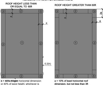
smaller, but not less than either 4% of least horizontal dimension or 3fASCE 7-16 ROOF ZONES
