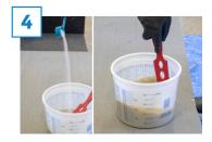
Using a slow-speed agitator, catalyze according to the mixing table and temperature on the product data sheet. Mix for an additional two (2) minutes. (Small amounts may also be hand-mixed.)
